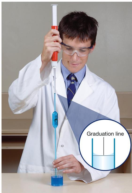
A pipette must always be filled using a safety pipette filler. When the pipette is filled correctly, the meniscus sits on the graduation line. Remember burette titres are read going DOWN.
